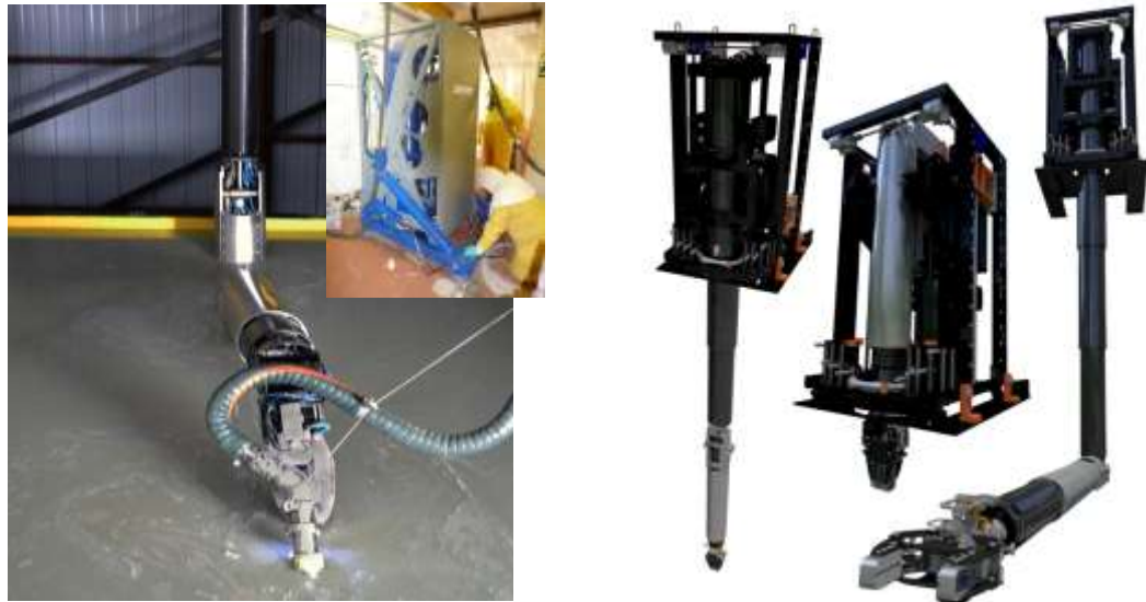
Figure 3 - Trawsfynydd Tank Cleaning Manipulator and Fukushima Inspection/Repair Manipulator
